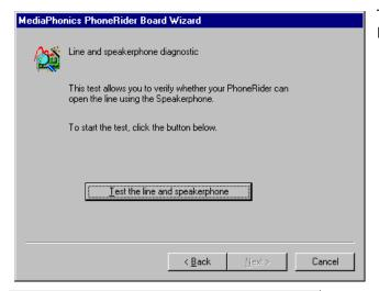
The **Line and Speakerphone Diagnostic** is displayed. Press the *Test the line and speakerphone* button.
