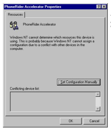
Then, the **PhoneRider Accelerator Properties** panel appears. Click the **Set Configuration Manually** button.
