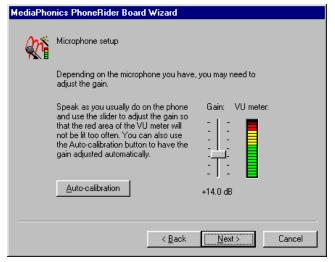
The **Microphone setup** panel appears. It allows you to finely adjust the microphone gain.
