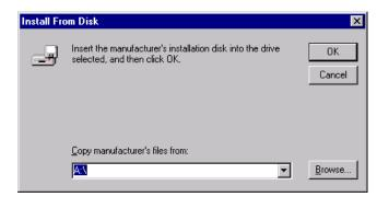
On the *Install From Disk* dialog box, click *Browse* or directly type in *C:\MPI2DRV*. If the path was entered the next panel will be *Select Device*.
