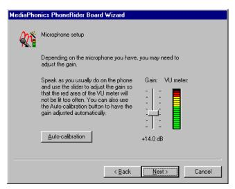
The **Microphone setup** panel appears. It allows you to finely adjust the microphone gain.
