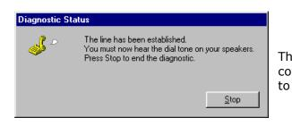
The **Diagnostic Status** window opens. If the board is correctly configured you can hear the card click. Click *Stop* to end the test.
